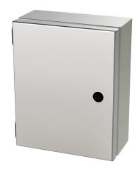
Saginaw Enviroline Junction series enclosure, NEMA 3R/4/4X/12/13, 10 x 8 x 4in (HxWxD), wall mount, 304 stainless steel, #4 brush finish, single-door, 1/4-turn semi-flush latch.
