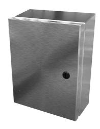
Saginaw Enviroline Junction series enclosure, slope top, NEMA 3R/4/4X/12/13,  $10 \times 8 \times 4$  in (HxWxD), wall mount, 304 stainless steel, #4 brush finish, single-door, 1/4-turn semi-flush latch.
