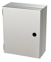
Saginaw Enviroline Junction series enclosure, NEMA 3R/4/4X/12/13, 10 x 8 x 4in (HxWxD), wall mount, 316L stainless steel, #4 brush finish, single-door, 1/4-turn semi-flush latch.
