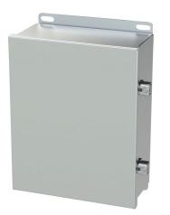
Saginaw enclosure, NEMA 3R/4/4X/12/13, 10 x 8 x 4in (HxWxD), wall mount, 304 stainless steel, #4 brush finish, single-door, stainless steel clamps.
