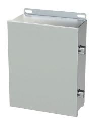
Saginaw enclosure, NEMA 3R/4/4X/12/13, 10 x 8 x 4in (HxWxD), wall mount, 316L stainless steel, #4 brush finish, single-door, stainless steel clamps.
