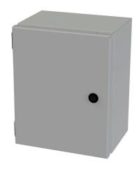
Saginaw Enviroline Junction series enclosure, NEMA 3R/4/12/13,  $10 \times 8 \times 6$  in (HxWxD), wall mount, carbon steel, ANSI 61 gray, powder coat finish, single-door, 1/4-turn semi-flush latch.
