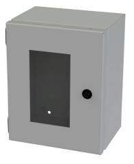
Saginaw Enviroline Junction series enclosure, NEMA 3R/4/12/13, 10 x 8 x 6in (HxWxD), wall mount, carbon steel, ANSI 61 gray, powder coat finish, single-door, 1/4-turn semi-flush latch, polycarbonate window.
