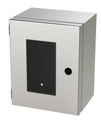
Saginaw Enviroline Junction series enclosure, NEMA 3R/4/4X/12/13,  $10 \times 8 \times 6$  in (HxWxD), wall mount, 304 stainless steel, #4 brush finish, single-door, 1/4-turn semi-flush latch, polycarbonate window.
