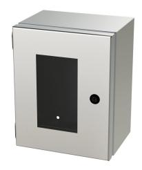
Saginaw Enviroline Junction series enclosure, NEMA 3R/4/4X/12/13,  $10 \times 8 \times 6$  in (HxWxD), wall mount, 316L stainless steel, #4 brush finish, single-door, 1/4-turn semi-flush latch, polycarbonate window.
