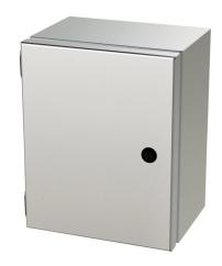
Saginaw Enviroline Junction series enclosure, NEMA 3R/4/4X/12/13, 10 x 8 x 6in (HxWxD), wall mount, 304 stainless steel, #4 brush finish, single-door, 1/4-turn semi-flush latch.
