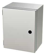
Saginaw Enviroline Junction series enclosure, NEMA 3R/4/4X/12/13, 10 x 8 x 6in (HxWxD), wall mount, 316L stainless steel, #4 brush finish, single-door, 1/4-turn semi-flush latch.
