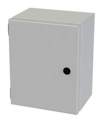
Saginaw Enviroline Junction series enclosure, NEMA 3R/4/12/13, 10 x 8 x 6in (HxWxD), wall mount, carbon steel, RAL 7035 light gray, powder coat finish, single-door, 1/4-turn semi-flush latch.
