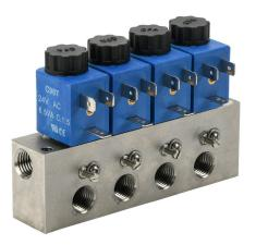
CFA solenoid valve bank, (4) stations, 2-port (2-way), N.C., 1/4in female NPT inlet(s), 1/4in female NPT outlet(s), Cv=0.14, individual metering, stainless steel body, 24 VAC, 6.5 VA, 11mm DIN style wiring plug.
