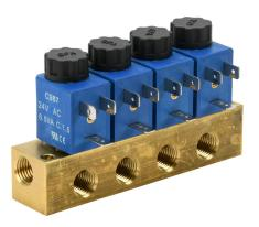
CFA solenoid valve bank, (4) stations, 2-port (2-way), N.C., 1/4in female NPT inlet(s), 1/4in female NPT outlet(s), Cv=0.14, brass body, 24 VAC, 6.5 VA, 11mm DIN style wiring plug.
