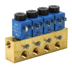
CFA solenoid valve bank, (4) stations, 2-port (2-way), N.C., 1/4in female NPT inlet(s), 1/4in female NPT outlet(s), Cv=0.14, individual metering, brass body, 24 VAC, 6.5 VA, 11mm DIN style wiring plug.
