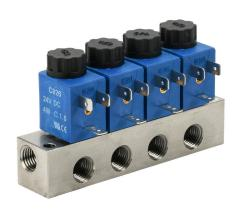
CFA solenoid valve bank, (4) stations, 2-port (2-way), N.C., 1/4in female NPT inlet(s), 1/4in female NPT outlet(s), Cv=0.14, stainless steel body, 24 VDC, 4W, 11mm DIN style wiring plug.
