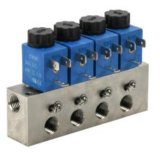
CFA solenoid valve bank, (4) stations, 2-port (2-way), N.C., 1/4in female NPT inlet(s), 1/4in female NPT outlet(s), Cv=0.14, individual metering, stainless steel body, 24 VDC, 4W, 11mm DIN style wiring plug.
