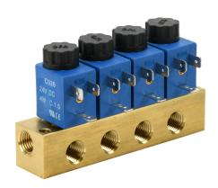
CFA solenoid valve bank, (4) stations, 2-port (2-way), N.C., 1/4in female NPT inlet(s), 1/4in female NPT outlet(s), Cv=0.14, brass body, 24 VDC, 4W, 11mm DIN style wiring plug.
