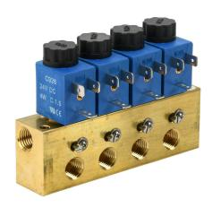
CFA solenoid valve bank, (4) stations, 2-port (2-way), N.C., 1/4in female NPT inlet(s), 1/4in female NPT outlet(s), Cv=0.14, individual metering, brass body, 24 VDC, 4W, 11mm DIN style wiring plug.
