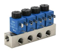
CFA solenoid valve bank, (4) stations, 2-port (2-way), N.C., 1/4in female NPT inlet(s), 1/4in female NPT outlet(s), Cv=0.14, stainless steel body, 120 VAC, 6.5 VA, 11mm DIN style wiring plug.
