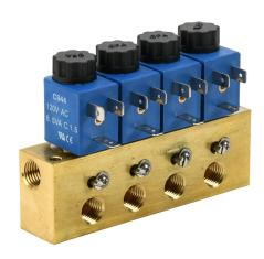
CFA solenoid valve bank, (4) stations, 2-port (2-way), N.C., 1/4in female NPT inlet(s), 1/4in female NPT outlet(s), Cv=0.14, individual metering, brass body, 120 VAC, 6.5 VA, 11mm DIN style wiring plug.
