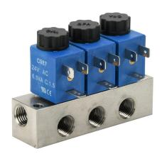
CFA solenoid valve bank, (3) stations, 2-port (2-way), N.C., 1/4in female NPT inlet(s), 1/4in female NPT outlet(s), Cv=0.14, stainless steel body, 24 VAC, 6.5 VA, 11mm DIN style wiring plug.
