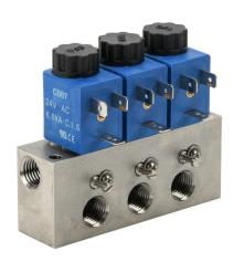
CFA solenoid valve bank, (3) stations, 2-port (2-way), N.C., 1/4in female NPT inlet(s), 1/4in female NPT outlet(s), Cv=0.14, individual metering, stainless steel body, 24 VAC, 6.5 VA, 11mm DIN style wiring plug.
