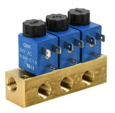
CFA solenoid valve bank, (3) stations, 2-port (2-way), N.C., 1/4in female NPT inlet(s), 1/4in female NPT outlet(s), Cv=0.14, brass body, 24 VAC, 6.5 VA, 11mm DIN style wiring plug.
