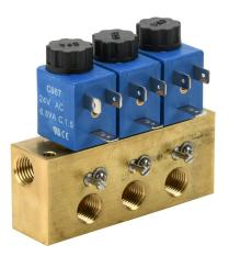
CFA solenoid valve bank, (3) stations, 2-port (2-way), N.C., 1/4in female NPT inlet(s), 1/4in female NPT outlet(s), Cv=0.14, individual metering, brass body, 24 VAC, 6.5 VA, 11mm DIN style wiring plug.
