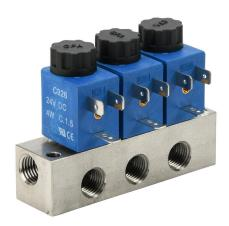
CFA solenoid valve bank, (3) stations, 2-port (2-way), N.C., 1/4in female NPT inlet(s), 1/4in female NPT outlet(s), Cv=0.14, stainless steel body, 24 VDC, 4W, 11mm DIN style wiring plug.
