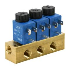
CFA solenoid valve bank, (3) stations, 2-port (2-way), N.C., 1/4in female NPT inlet(s), 1/4in female NPT outlet(s), Cv=0.14, brass body, 24 VDC, 4W, 11mm DIN style wiring plug.
