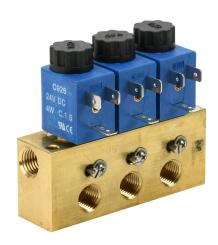
CFA solenoid valve bank, (3) stations, 2-port (2-way), N.C., 1/4in female NPT inlet(s), 1/4in female NPT outlet(s), Cv=0.14, individual metering, brass body, 24 VDC, 4W, 11mm DIN style wiring plug.
