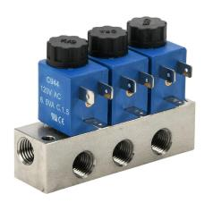
CFA solenoid valve bank, (3) stations, 2-port (2-way), N.C., 1/4in female NPT inlet(s), 1/4in female NPT outlet(s), Cv=0.14, stainless steel body, 120 VAC, 6.5 VA, 11mm DIN style wiring plug.
