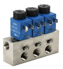
CFA solenoid valve bank, (3) stations, 2-port (2-way), N.C., 1/4in female NPT inlet(s), 1/4in female NPT outlet(s), Cv=0.14, individual metering, stainless steel body, 120 VAC, 6.5 VA, 11mm DIN style wiring plug.
