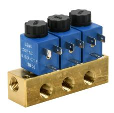
CFA solenoid valve bank, (3) stations, 2-port (2-way), N.C., 1/4in female NPT inlet(s), 1/4in female NPT outlet(s), Cv=0.14, brass body, 120 VAC, 6.5 VA, 11mm DIN style wiring plug.
