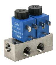
CFA solenoid valve bank, (2) stations, 2-port (2-way), N.C., 1/4in female NPT inlet(s), 1/4in female NPT outlet(s), Cv=0.14, stainless steel body, 24 VAC, 6.5 VA, 11mm DIN style wiring plug.
