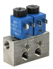
CFA solenoid valve bank, (2) stations, 2-port (2-way), N.C., 1/4in female NPT inlet(s), 1/4in female NPT outlet(s), Cv=0.14, individual metering, stainless steel body, 24 VAC, 6.5 VA, 11mm DIN style wiring plug.
