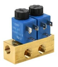
CFA solenoid valve bank, (2) stations, 2-port (2-way), N.C., 1/4in female NPT inlet(s), 1/4in female NPT outlet(s), Cv=0.14, brass body, 24 VAC, 6.5 VA, 11mm DIN style wiring plug.
