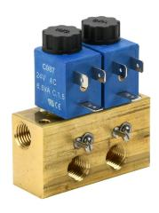
CFA solenoid valve bank, (2) stations, 2-port (2-way), N.C., 1/4in female NPT inlet(s), 1/4in female NPT outlet(s), Cv=0.14, individual metering, brass body, 24 VAC, 6.5 VA, 11mm DIN style wiring plug.
