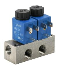
CFA solenoid valve bank, (2) stations, 2-port (2-way), N.C., 1/4in female NPT inlet(s), 1/4in female NPT outlet(s), Cv=0.14, stainless steel body, 24 VDC, 4W, 11mm DIN style wiring plug.
