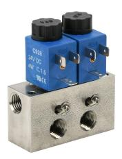
CFA solenoid valve bank, (2) stations, 2-port (2-way), N.C., 1/4in female NPT inlet(s), 1/4in female NPT outlet(s), Cv=0.14, individual metering, stainless steel body, 24 VDC, 4W, 11mm DIN style wiring plug.
