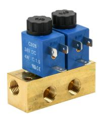
CFA solenoid valve bank, (2) stations, 2-port (2-way), N.C., 1/4in female NPT inlet(s), 1/4in female NPT outlet(s), Cv=0.14, brass body, 24 VDC, 4W, 11mm DIN style wiring plug.
