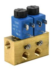
CFA solenoid valve bank, (2) stations, 2-port (2-way), N.C., 1/4in female NPT inlet(s), 1/4in female NPT outlet(s), Cv=0.14, individual metering, brass body, 24 VDC, 4W, 11mm DIN style wiring plug.
