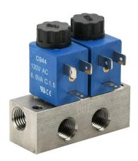
CFA solenoid valve bank, (2) stations, 2-port (2-way), N.C., 1/4in female NPT inlet(s), 1/4in female NPT outlet(s), Cv=0.14, stainless steel body, 120 VAC, 6.5 VA, 11mm DIN style wiring plug.
