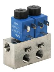
CFA solenoid valve bank, (2) stations, 2-port (2-way), N.C., 1/4in female NPT inlet(s), 1/4in female NPT outlet(s), Cv=0.14, individual metering, stainless steel body, 120 VAC, 6.5 VA, 11mm DIN style wiring plug.
