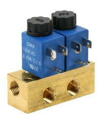
CFA solenoid valve bank, (2) stations, 2-port (2-way), N.C., 1/4in female NPT inlet(s), 1/4in female NPT outlet(s), Cv=0.14, brass body, 120 VAC, 6.5 VA, 11mm DIN style wiring plug.
