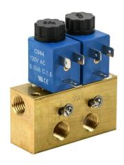
CFA solenoid valve bank, (2) stations, 2-port (2-way), N.C., 1/4in female NPT inlet(s), 1/4in female NPT outlet(s), Cv=0.14, individual metering, brass body, 120 VAC, 6.5 VA, 11mm DIN style wiring plug.
