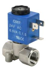
CFA solenoid valve, 3-port (3-way), 2-position, N.C., stainless steel body, Viton seal(s), 1/4in female NPT inlet(s), 1/4in female NPT outlet(s), Cv=0.084, 0 psi minimum operating pressure, 24 VAC operating voltage, 11mm DIN style wiring plug.
