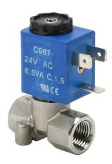
CFA solenoid valve, 3-port (3-way), 2-position, N.C., stainless steel body, Viton seal(s), 1/4in female NPT inlet(s), 1/4in female NPT outlet(s), Cv=0.084, 0 psi minimum operating pressure, 24 VAC operating voltage, 11mm DIN style wiring plug.
