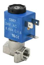
CFA solenoid valve, 3-port (3-way), 2-position, N.C., stainless steel body, Viton seal(s), 1/8in female NPT inlet(s), 1/8in female NPT outlet(s), Cv=0.084, 0 psi minimum operating pressure, 24 VAC operating voltage, 11mm DIN style wiring plug.
