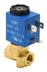
CFA solenoid valve, 3-port (3-way), 2-position, N.C., brass body, Viton seal(s), 1/8in female NPT inlet(s), 1/8in female NPT outlet(s), Cv=0.084, 0 psi minimum operating pressure, 24 VAC operating voltage, 11mm DIN style wiring plug.
