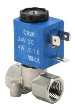
CFA solenoid valve, 3-port (3-way), 2-position, N.C., stainless steel body, Viton seal(s), 1/4in female NPT inlet(s), 1/4in female NPT outlet(s), Cv=0.084, 0 psi minimum operating pressure, 24 VDC operating voltage, 11mm DIN style wiring plug.
