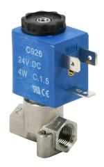
CFA solenoid valve, 3-port (3-way), 2-position, N.C., stainless steel body, Viton seal(s), 1/8in female NPT inlet(s), 1/8in female NPT outlet(s), Cv=0.084, 0 psi minimum operating pressure, 24 VDC operating voltage, 11mm DIN style wiring plug.
