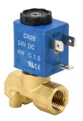
CFA solenoid valve, 3-port (3-way), 2-position, N.C., brass body, Viton seal(s), 1/4in female NPT inlet(s), 1/4in female NPT outlet(s), Cv=0.084, 0 psi minimum operating pressure, 24 VDC operating voltage, 11mm DIN style wiring plug.
