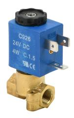
CFA solenoid valve, 3-port (3-way), 2-position, N.C., brass body, Viton seal(s), 1/8in female NPT inlet(s), 1/8in female NPT outlet(s), Cv=0.084, 0 psi minimum operating pressure, 24 VDC operating voltage, 11mm DIN style wiring plug.
