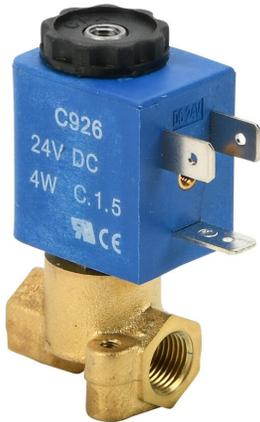
CFA solenoid valve, 3-port (3-way), 2-position, N.C., brass body, Viton seal(s), 1/8in female NPT inlet(s), 1/8in female NPT outlet(s), Cv=0.084, 0 psi minimum operating pressure, 24 VDC operating voltage, 11mm DIN style wiring plug.
